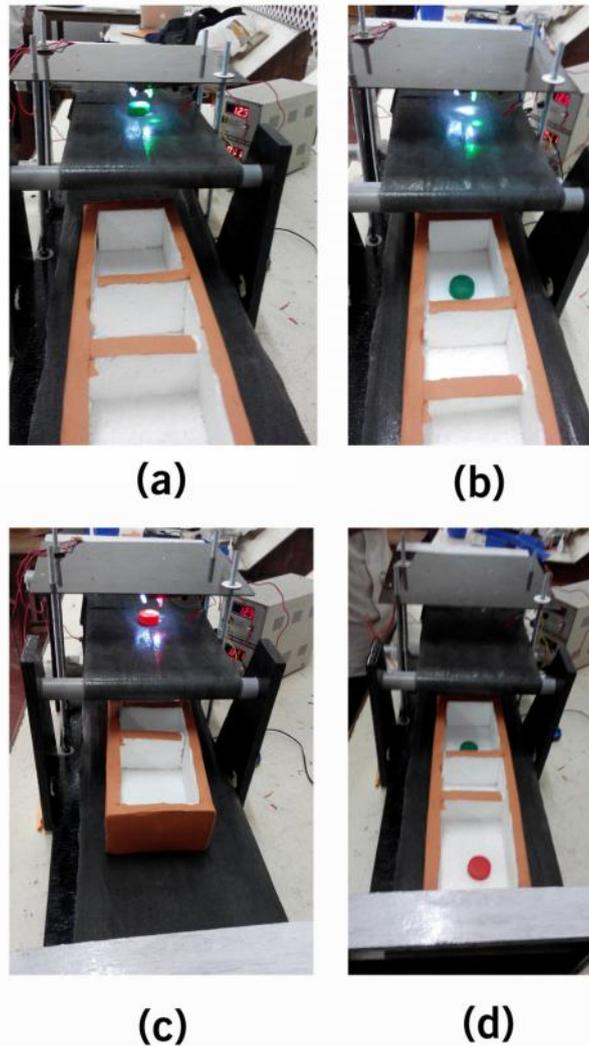
**Figure 4:** (a)The color sensor identifying the color of object 1, (b)the object 1 (Green) falls into the first section of the container, (c) The color sensor identifying the color of object 2, and (d)the object 2 (Red) falls into the third section of the container.
